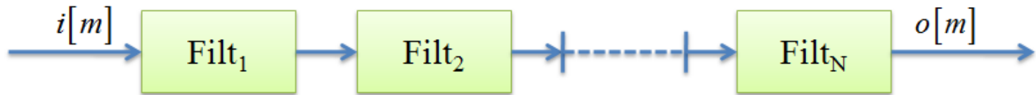
Figure 2: Scheme for serial filtering. The output of each filter is input to the following filter till the end of the series.
