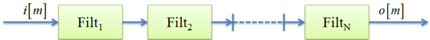
Figure 2: Scheme for serial filtering. The output of each filter is input to the following filter till the end of the series.
